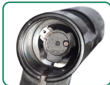
Fig.7: Extractor protrudes beyond the outer edge of the bolt
